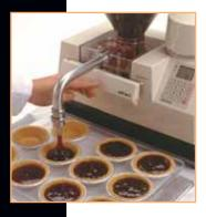
PV-Series The PV-Series power base gives the operator complete control over the speed at which a product is dispensed
