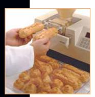
All power bases can be triggered manually by a trip arm (standard on P, PS, PV or PT power bases), our foot switch or hose assembly (accessories), or your own photoelectric switch.
