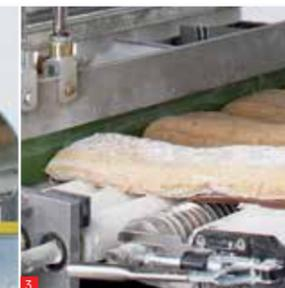
5 After rounding, a range of stamping tools can be used to shape a wide range of bread varieties.
