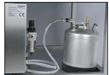
Compressed air connection and 9l oil tank
