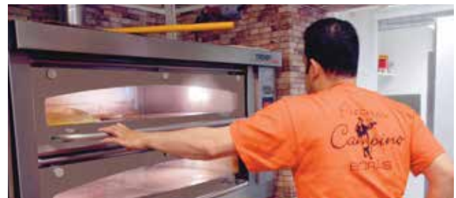
Double side halogen lighting. Oven doors with heat-reflecting toughened glass.
