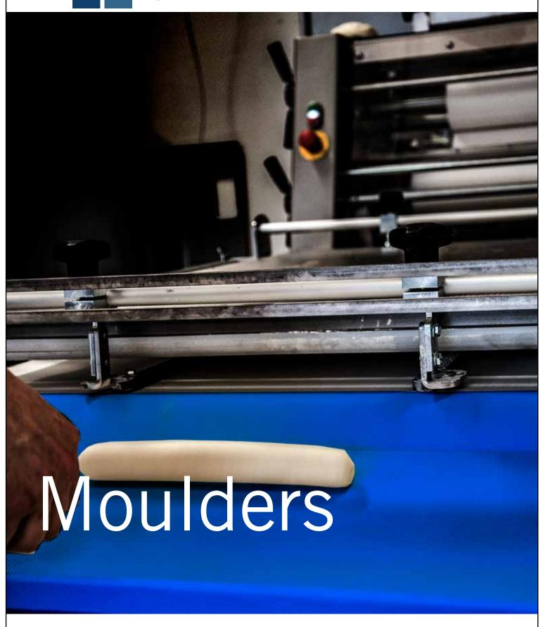
Moulder with capacity up to 3000 pieces/hour and weight range 30-1800 g.
