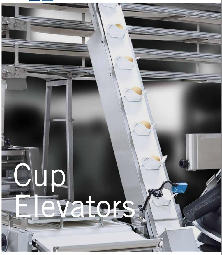
Cup Elevator with capacity up to 2000 pieces/hour. Weight range between 100-1500 grams.
