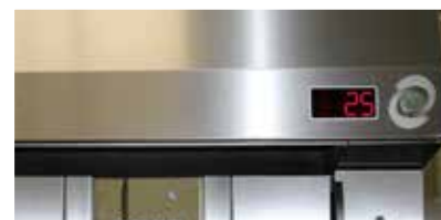
Practical remote display for display of the remaining baking time
