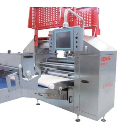
The TwinSat's function is based on a sophisticated system. By positioning two satellite roller heads one above the other, it is possible to produce virtually tension-free dough.
