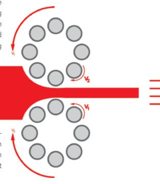
The major difference to ordinary satellite systems with standard cylindrical rollers lies in the twin satellite head which reduces high mechanical loads on the dough to a minimum and largely restricts dough tension. We call this the TwinSat principle.
