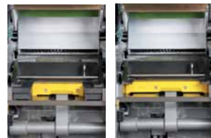
Adjustment from 5-row operation to 3-row operation.
