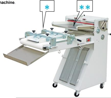
\*To use sheeter feature: remove dough roller/ pressure plate mounting system and rolling chain.
